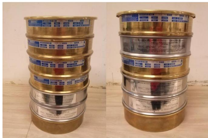
FIGURA 4 – ENSAIO GRANULOMÉTRICO: (A) AREIA E (B) BRITA.
