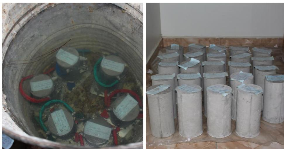
FIGURA 2 – (A) CORPOS DE PROVA EM CURA POR IMERSÃO / (B) CORPOS DE PROVA DESFORMADOS, EM CURA AO AR LIVRE.
