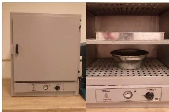
FIGURA 5 – ENSAIO: MATERIAL PULVERULENTO (ESTUFA).
