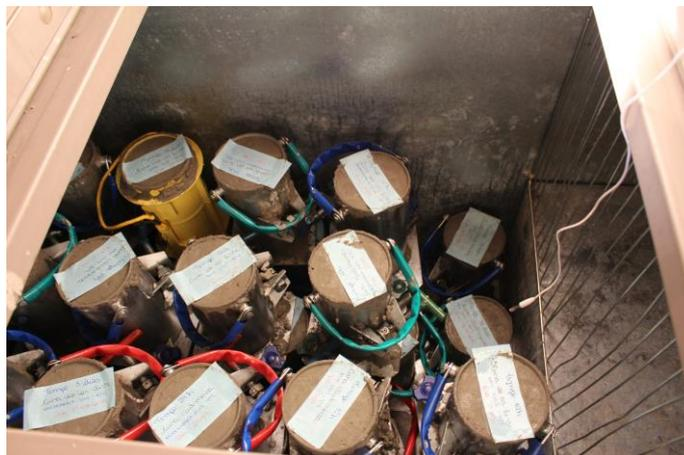
FIGURA 1 – CORPOS DE PROVA EXPOSTOS A BAIXA TEMPERATURA.
