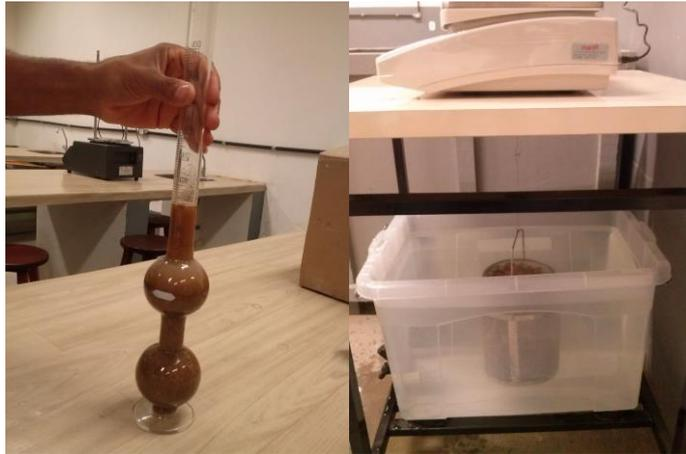
FIGURA 3 – ENSAIO DA MASSA ESPECÍFICA: AREIA (A) E DA BRITA (B).
