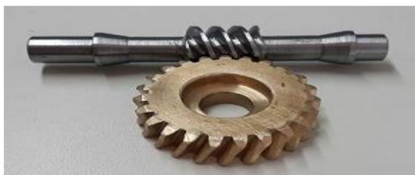
FIGURA 6: COROA E PARAFUSO SEM-FIM PROJETADO PELA EQUIPE
